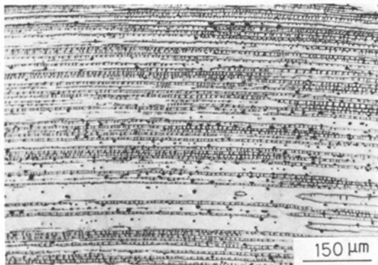
Figure 10 5143 filament wire reacted for three days at 700° C and drawn 10%; longitudinal section.
